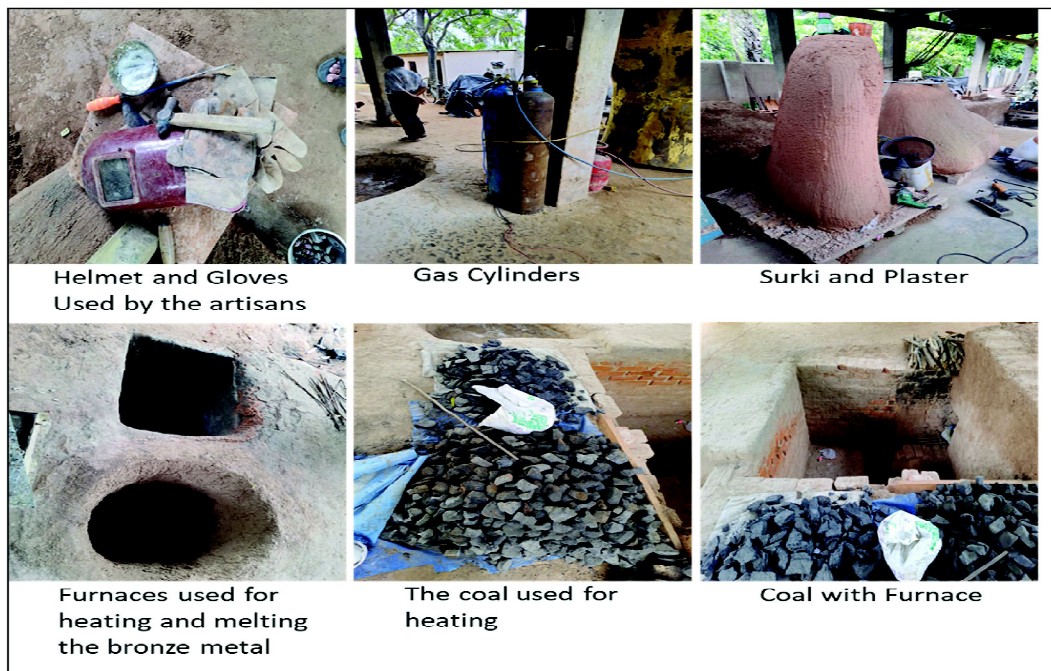
Fig. 5: Infrastructure and equipment used for bronze casting. (Captured by the author on August 27, 2025, Ghurni, Krishnanagar, West Bengal, India)
